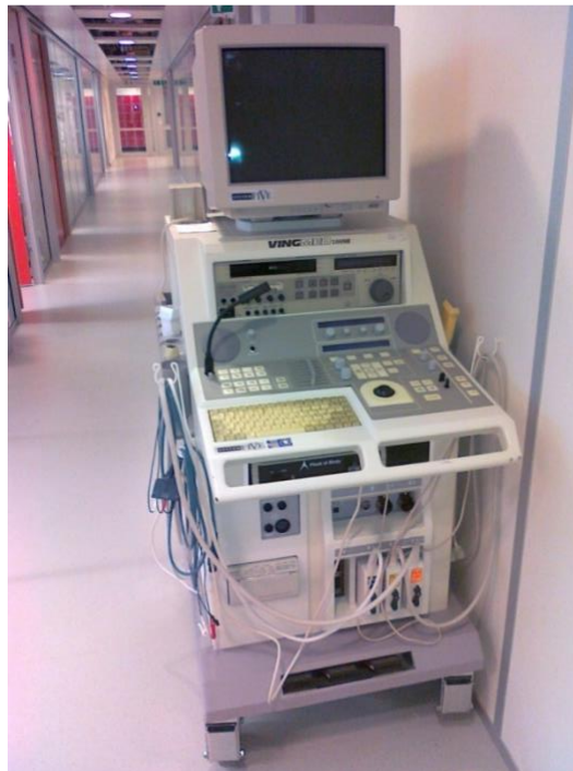
Figure 3 System 5. The first ultrasound scanner from Vingmed with electronic probes.
