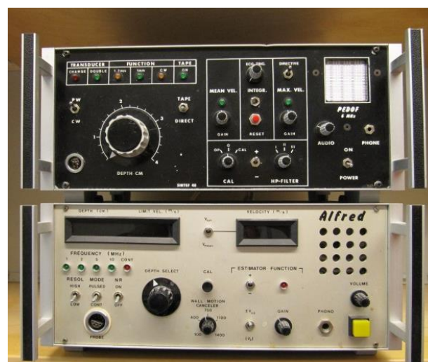
Figure 1 Doppler Instruments. The 1976 PEDOF (top) and 1980 ALFRED (bottom) Doppler prototypes developed in Trondheim.
