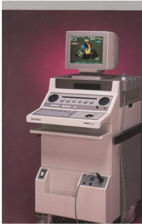
Figure 2 Vingmed CFM700. The first ultrasound scanner developed and manufactured in Norway, the Vingmed CFM700 annular array scanner.
